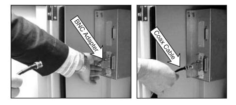
Figure 1-6. Connecting with the BNC adapter.
