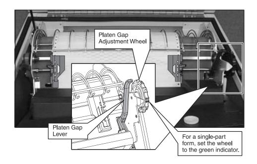
Figure 1–10. Platen Gap Adjustment Wheel and Lever
