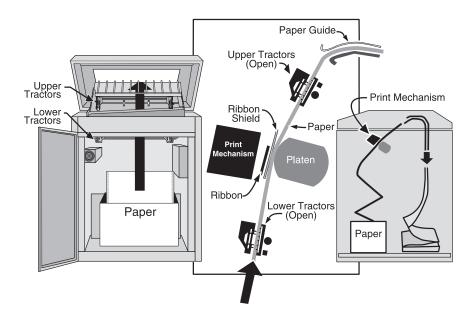
Figure 1–15. Paper Box Placement and Paper Path
