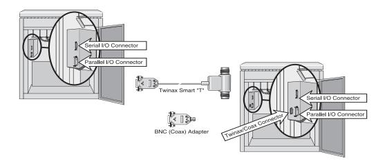
Figure 1-4. Serial/Parallel and FourPlex Interface Connectors (Rear View)
