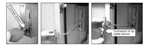
Figure 1-5. Connecting the Host Connector Smart T
