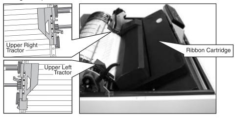
Figure 1–8. Paper System Components
