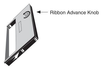
Figure 1–12. Removing Ribbon Slack
