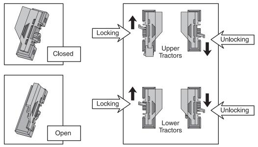
Figure 1–9. Opening, Locking, and Unlocking Tractors
