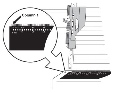
Figure 1–16. Column Alignment Scale
