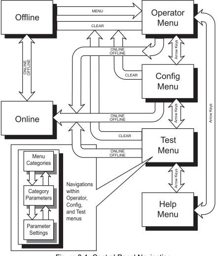
Figure 3-1 Control Panel Navigation
