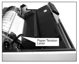
Figure 1–11. Paper Tension Lever
