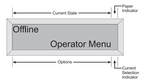
Figure 2-2. Control Panel Display
