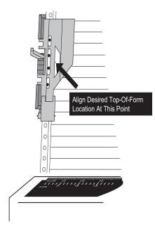
Figure 2-3 . Aligning Form on Tractors
